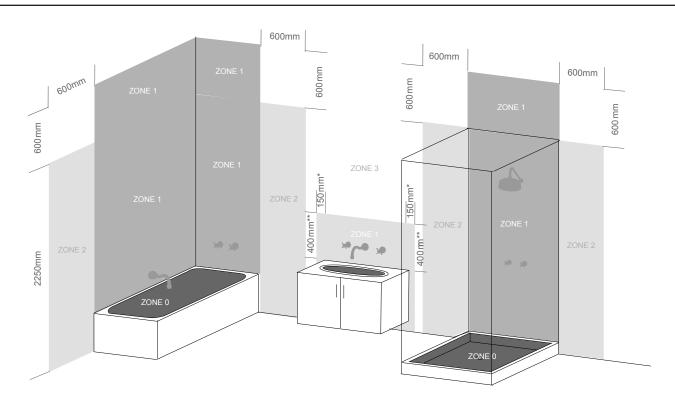
HAWTHORN HILL TOWEL WARMERS HAVE AN IP RATING OF IP55 ALLOWING INSTALLATION INTO ZONES 1, 2, AND 3.
